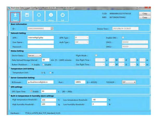
**Step7:** Set the APN of the SIM card, the platform IP address and port for uploading data, the sending interval, the GPS opening time and other information, and click "Save" after setting.
